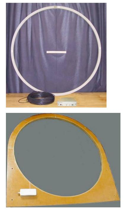
The above left picture shows the four arc segments of a similar system's rotating Transmitter. The middle picture shows the assembled picture for that same system, along with an AT-4400 Receiver and a lengthy Pickup-to-Receiver coaxial cable. The picture on the right shows a typical stationary induction power/data pickup for large diameter shafts.
